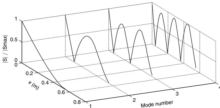
Figure 2: Normalized sensitivity functions for the rectangle-shaped piezoelectric sensor attached to a cantilevered beam of length 58 cm as a function of the structural mode number and the distance of the sensor from the clamped end of the beam.
