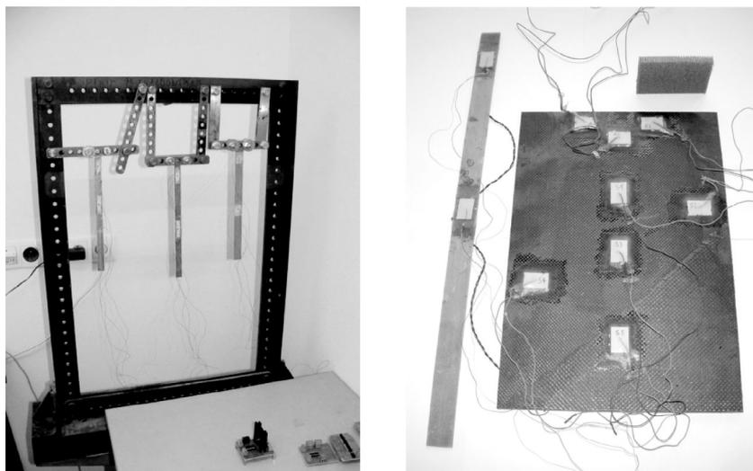
Figure 3: Three thin aluminium beams fixed to an experimental stand (left); a glass-fiber composite beam and a sandwich panel made up from the carbon-fiber composite liners with the Nomex-honeycomb core (right) used in experimental investigations.
