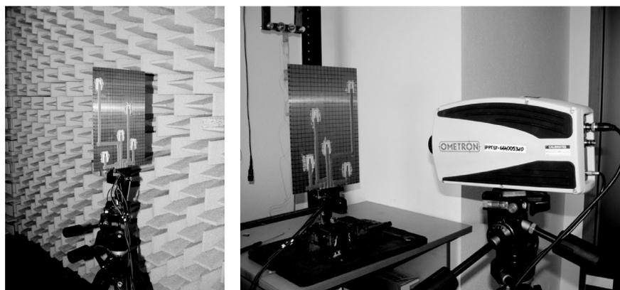
Figure 5: Thin aluminium plate with attached piezoelectric transducers in laboratory stands used in experimental investigations.
