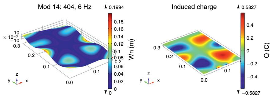
Figure 4: Results of the numerical simulations: the shape of an exemplary vibrational mode of the considered plate structure made of aluminium (left) and the corresponding distribution of the induced electric charge induced on the theoretical point-sensors made of the considered piezoceramics (right).
