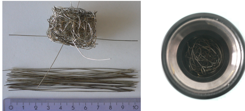
Figure 1: Manufacturing of a fibrous sample from 10 cm long pieces of copper wire with diameter 0.5 mm, and the sample inside the impedance tube with diameter 29 mm
