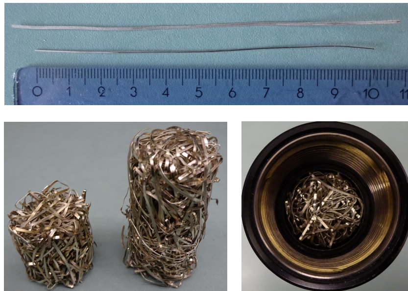
Figure 16: A piece of oblate wire (with its rounded original below) and two fibrous samples with porosity 90% (one of the samples is shown also inside the impedance tube)
