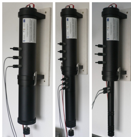
Figure 2: Three vertically-positioned impedance tubes
