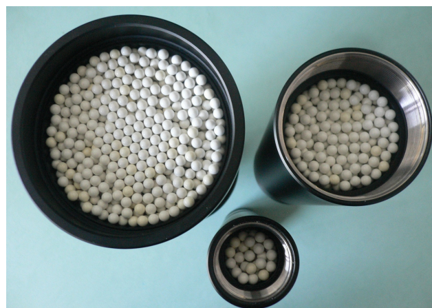
Figure 1: Randomly-packed spherical beads inside three tubes of various size
