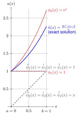
One can check that this approximation is in fact the exact solution. Such result is obtained thanks to the choice of shape functions (the simple subspace generated by the shape functions happens to contain the exact solution).
