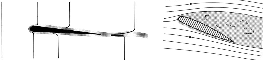
**FIGURE 7:** Flows past an airfoil: [left] unseparated flow at small angle of attack (the fate of successive lines of fluid particles is shown), [right] a separated flow at large angle of attack (the layer separation is responsible for the sudden drop in lift).
