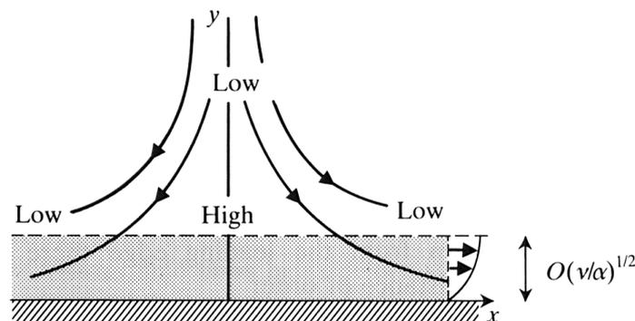
**FIGURE 5:** A two-dimensional flow towards a stagnation point.
