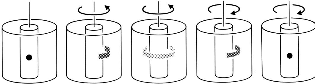
**FIGURE 2:** Reversibility of a very viscous flow.
