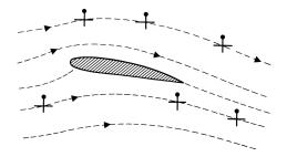
■ There are **no regions of closed streamlines** in the flow; all the streamlines can be traced back to  $-\infty$ .
