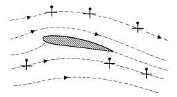
**Steady flow** past a wing at **small angle of attack** (incidence) is typically **irrotational**.
