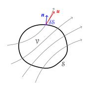
Now, using the divergence theorem and the assumption of the "smoothness" of flow (i.e., continuous velocity gradient) gives the condition for incompressible flow.
