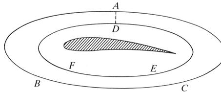
$$\begin{aligned} 0 &= \Gamma_{ABCADEFDA} \\ &= \Gamma_{ABCA} + \Gamma_{AD} + \Gamma_{DEFD} + \Gamma_{DA} \\ &= \Gamma_{ABCA} + \Gamma_{AD} - \Gamma_{DFED} - \Gamma_{AD} \quad \longrightarrow \quad \Gamma_{ABCA} = \Gamma_{DFED} \end{aligned}$$
