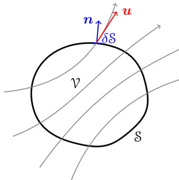
**FIGURE 2:** Flow through a closed surface
