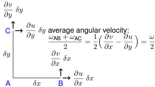
**FIGURE 3:** Interpretation of vorticity in 2D flow. The velocity components are relative to the fluid particle at A.
