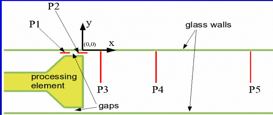
Schematic view of the emulsifier with coordinates system and positions of selected profiles
