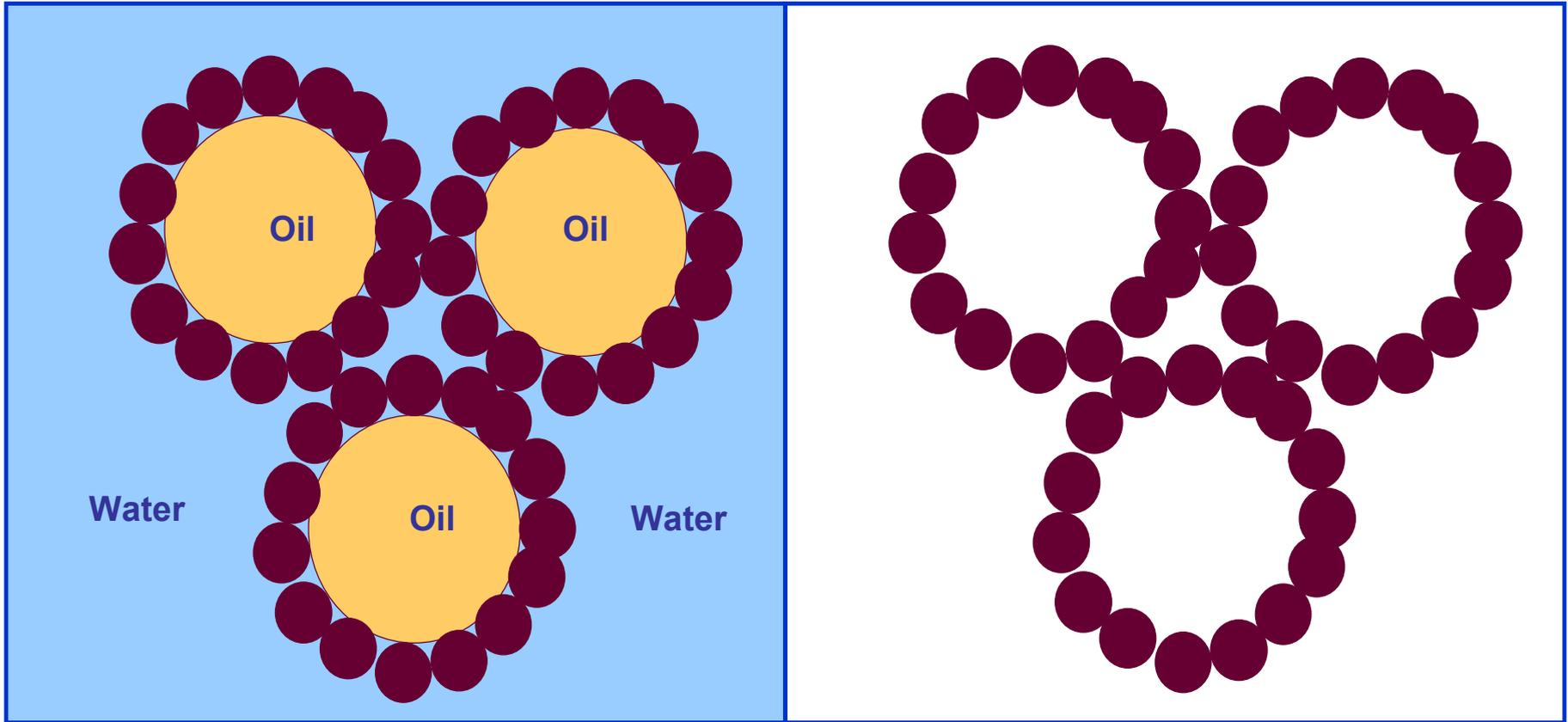
The emulsion with thin layers of third substance at the surface between oil and water
