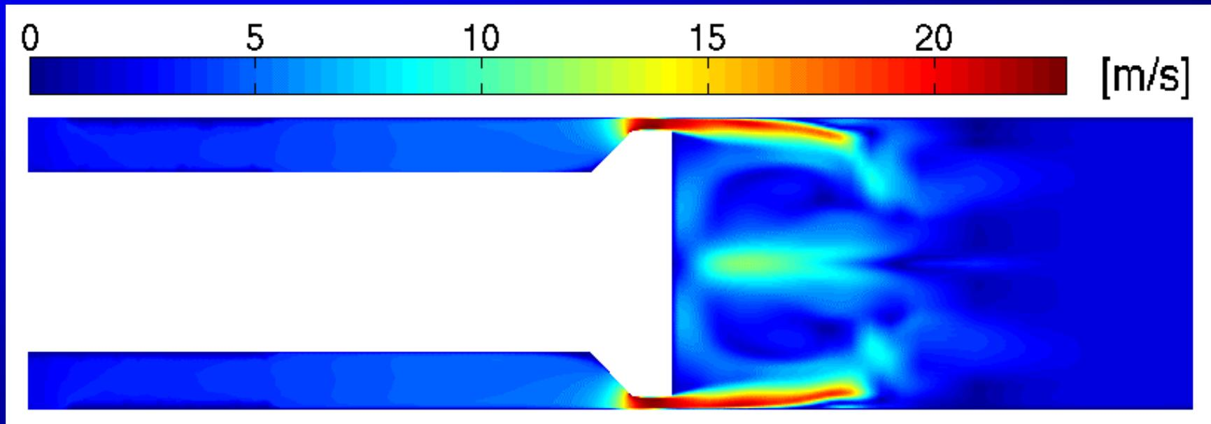
Laminar – unsteady flow,  $Q_2 = 0.204 \text{ dm}^3/\text{s}$
