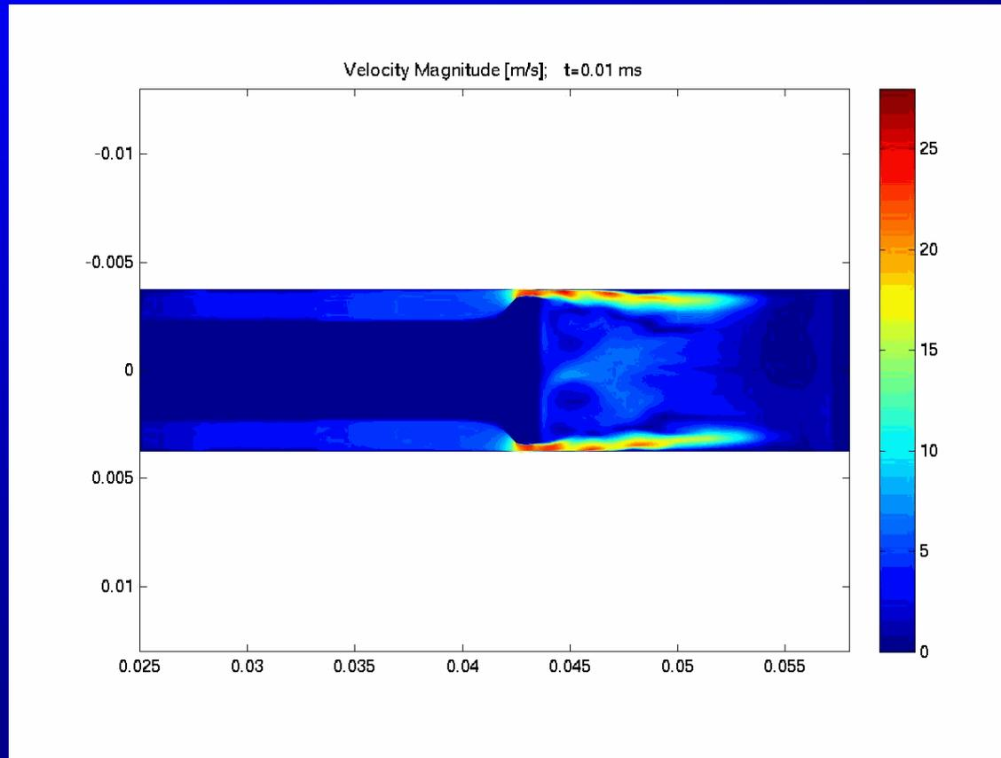
Laminar – unsteady flow,  $Q_2 = 0.204 \text{ dm}^3/\text{s}$
