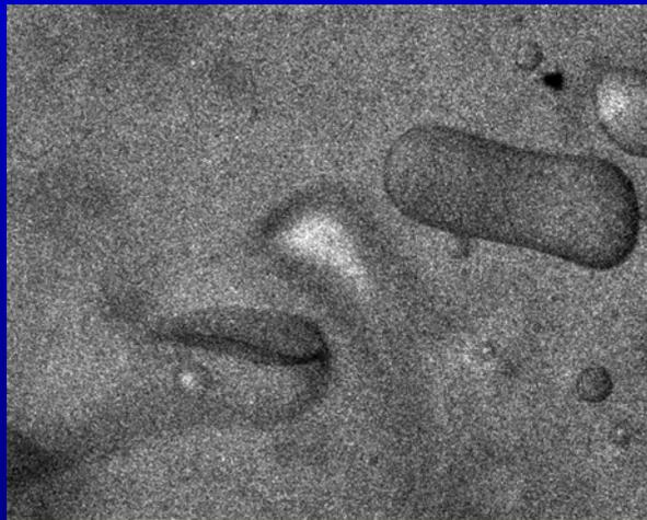
**Deformed drops of S50 silicone oil
