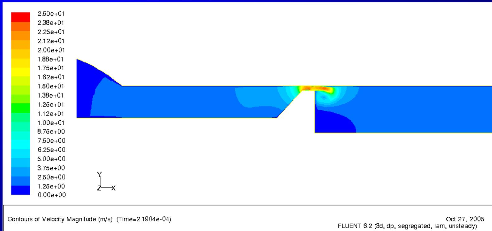
Laminar – unsteady flow,  $Q_2 = 0.204 \text{ dm}^3/\text{s}$
