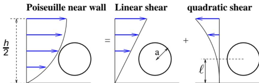
$$u(z) = k_s z + k_q z^2 \quad \text{where: } k_s = \frac{h}{2\mu_f} \left( -\frac{dp}{dx} \right), \quad k_q = \frac{1}{2\mu_f} \left( \frac{dp}{dx} \right).$$
