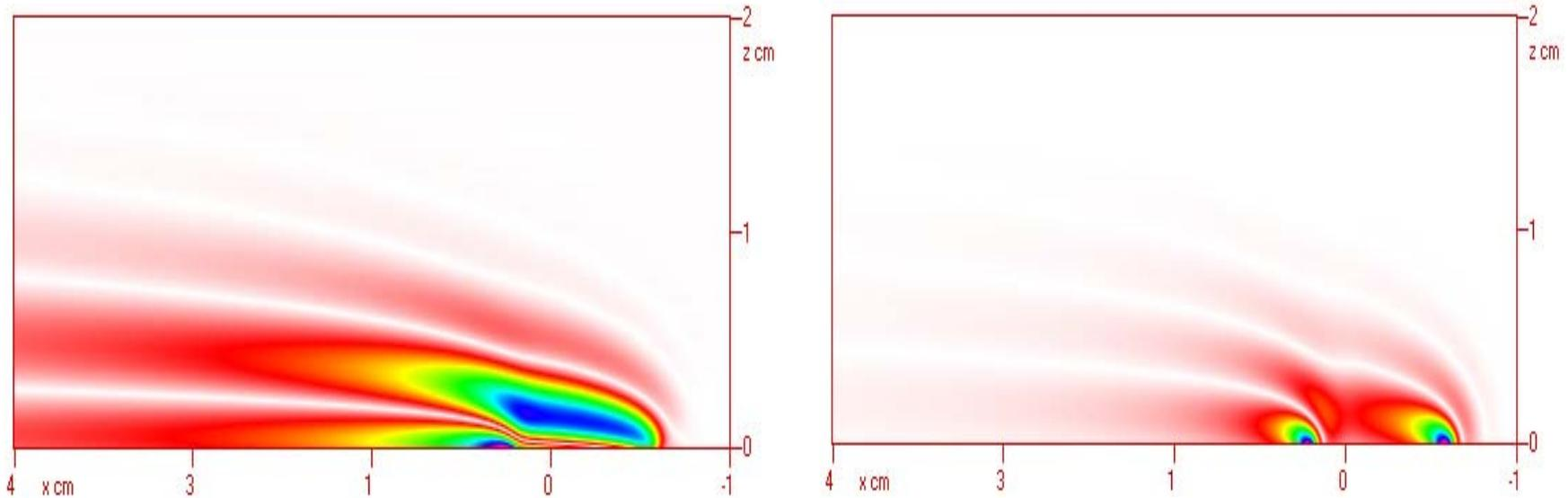
Slowly moving strip *a, b*) horizontal and vertical velocity components
