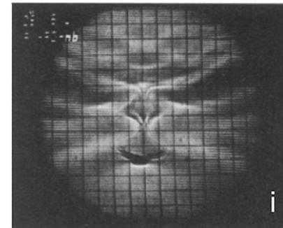
Intersection of two periodic internal wave beams produced by independent sources
