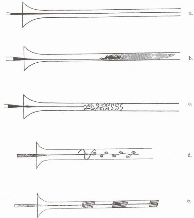
Reynolds' drawings of kinds of flow in a tube, as indicated by the ink jet method. "Direct" flow (a), "sinuous" flow (b), the same observed with a flash of light (c), disturbance of direct flow by a wire (d), intermittent "flashes" of eddying (e). *Source:* Reynolds (ref. 100), 59, 60, 76, 77.
