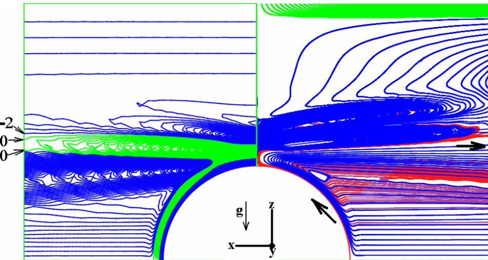
Interferometric image of diffusion induced flow on a gas bubble in a stratified solution of acetic acid
