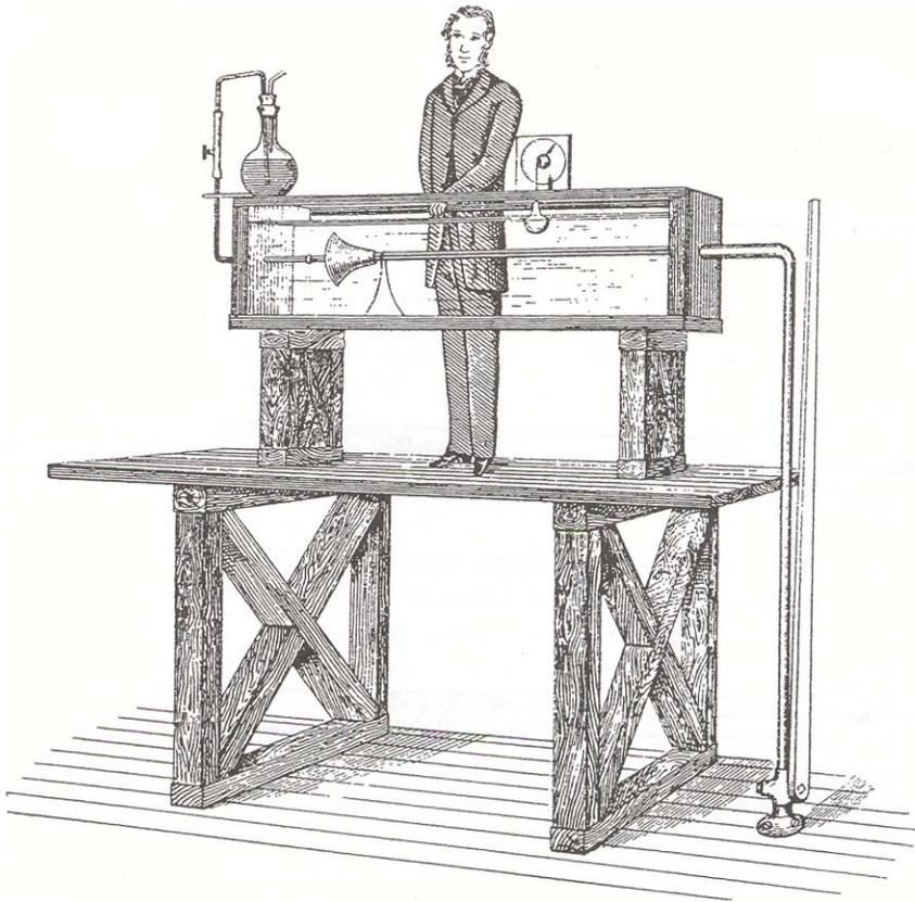
Reynolds' apparatus for studying the turbulent transition of the flow of water in a tube. Water from the tank enters the horizontal glass tube through the conical funnel. The valve with the long handle on the right controls the flux, whose value is inferred from the lowering of the floater. Ink from the flask is injected continuously in the middle of the entrance of the tube. *Source:* Reynolds (ref. 100), 71.
