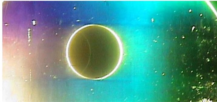
**Diffusion induced flow formation on a motionless sphere submerged in exponentially stratified fluid at rest**
