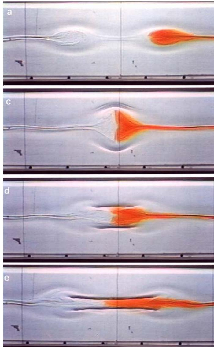
Collision of solitons on the interface between miscible fluids
