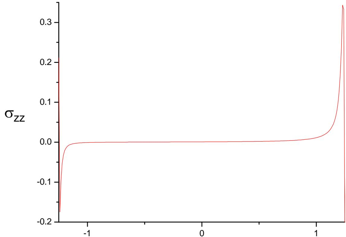
$$\sigma_{zz}(x, z, t) = \frac{i\nu U}{\pi} \int_{-\infty}^{\infty} \sin \frac{ka}{2} e^{ik(x-Ut)} \frac{k_w(kU, k) e^{ik_w(kU, k)z} - k_i(kU, k) e^{ik_i(kU, k)z}}{k_w(kU, k) - k_i(kU, k)} dk$$
