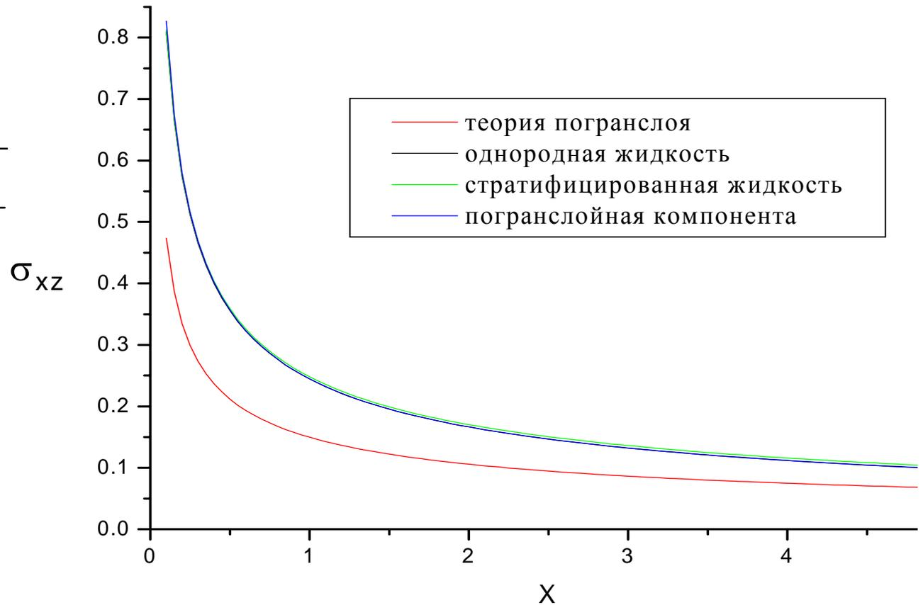
$$\sigma_{xz}(x, z, t) = -\frac{i\nu U}{\pi} \int_{-\infty}^{\infty} \frac{1}{k} \sin \frac{ka}{2} e^{ik(x-Ut)} \frac{k_w^2(kU, k) e^{ik_w(kU, k)z} - k_i^2(kU, k) e^{ik_i(kU, k)z}}{k_w(kU, k) - k_i(kU, k)} dk$$
