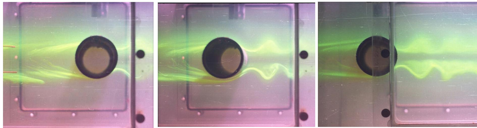
Re-distribution of a released dye ahead and past the cylinder and formation of bright envelopes on a high gradient interfaces inside the density wake ( $D = 7.6$  см;  $T_b = 7$ . s;  $U = 0.69$  см/с;  $Fr = 0.1$ ;  $Re = 524$ ).
