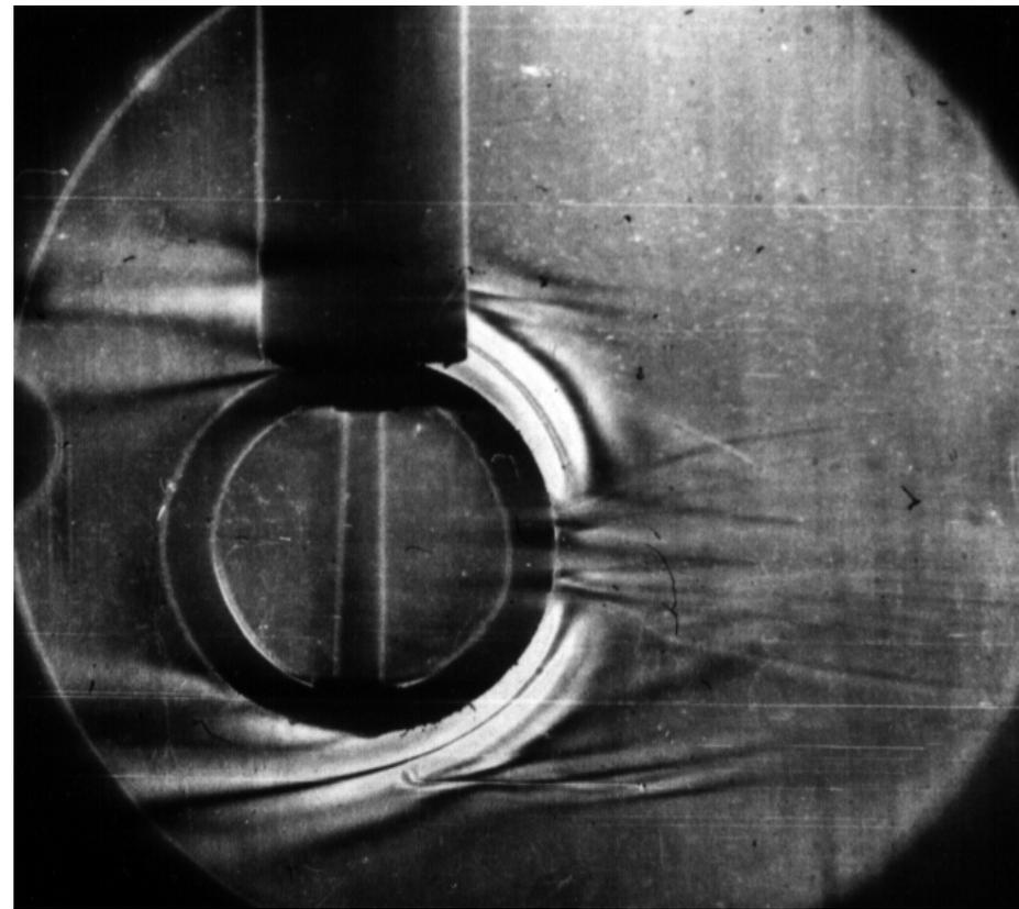
Conventional (left) and Maksoutov (right) schlieren images of the flow past a cylinder;
