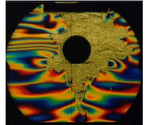
Colour images of “natural rainbow” schlieren image of the flow with auto cumulative jets around sphere ( $D = 4.5$  cm,  $T_b = 7,9$  c,  $H = 12$  cm): *a, b*) – sinking and first rising of the sphere; *c, d*) and *e, f*) – forming the first and decaying the second jets
