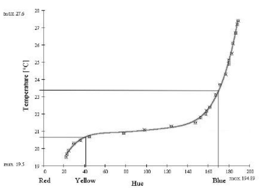
Figure 4: Calibration curve for KXN 2030 liquid crystals
