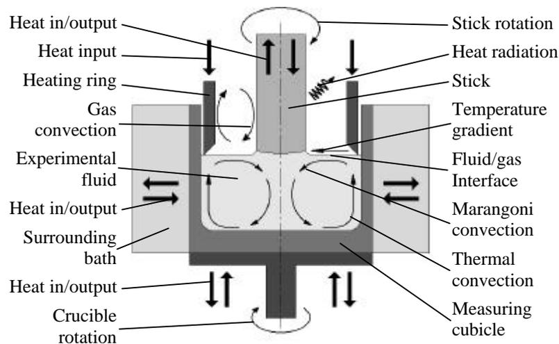
Figure 1: Schema of the modified Czochralski configuration
