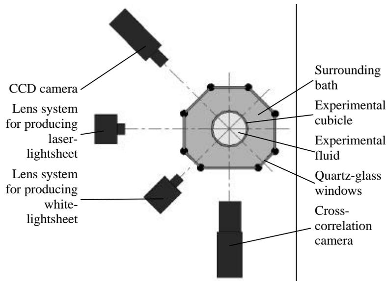
Figure 2: Lightsheet systems layout of the experimental equipment
