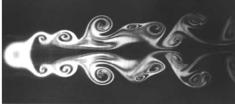
Fig. 3. Visualization of the vortices forming in the shear layer between the jet and the cross stream. The plane of the photo is parallel to the wall where the jet is flush mounted; velocity ratio R = 2 .
