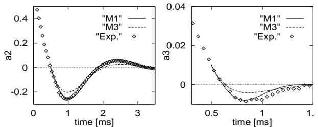
Figure 4: Oscillations amplitude  $a_2$  and  $a_3$  measured for a glycerin-water mixture (points);  $R_0 = 417\mu$ ,  $Re = 3.3$ . Comparison with nonlinear model M1 (solid line) and linear model M3.
