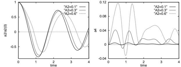
Figure 8: Effect of deformation amplitude. Numerical simulation using model M1,  $Re = 33$ , initial conditions:  $a_2 = 0.1, 0.3, 0.6$ ,  $\dot{a}_2 = 0$ , and all remaining modes set to zero; (right) - normalized amplitude  $a_2$ , (left) - excited amplitude  $a_4$ .
