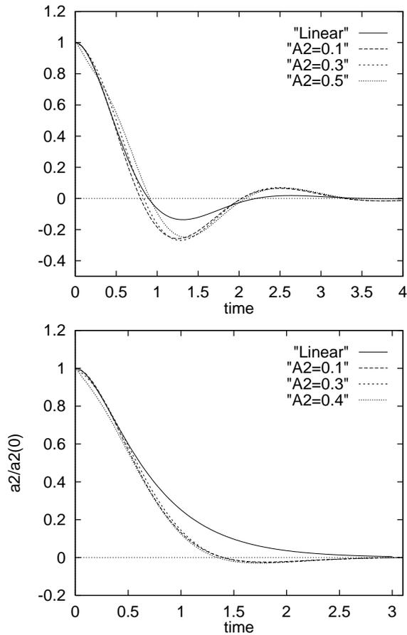
Figure 9: Effect of deformation amplitude for near aperiodic limit. Linear model M3 and simulation using model M1 at three different initial deformations; (top)-  $Re = 3.3$  - case to be compared with Fig.4 in [4], (bottom)-  $Re = 1.67$  - case to be compared with Fig.3 in [4].
