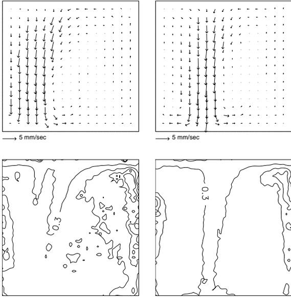
Figure 4: Measured development of the flow structure.  $Ra = 2.7 \times 10^6$ ,  $T_h = 21^\circ C$ ,  $T_c = 15.5^\circ C$ . Velocity vectors and non-dimensional temperature distribution at the vertical centre plane  $z=0.5$ .
