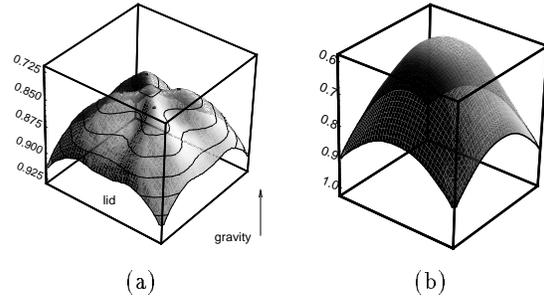
Figure 9: *Ice formation under the lid of the lid-cooled cavity. Ice surface calculated at 6 min (a) and 60 min (b) after the start of cooling started. The interface is seen from below.  $Ra = 3.1 \times 10^6$ ,  $Pr = 13$ .*
