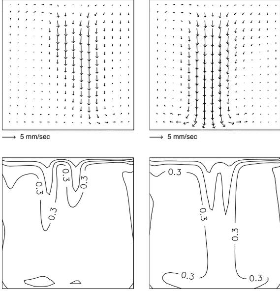
Figure 3: Numerical simulation of the development of the flow structure.  $Ra = 2.7 \times 10^6$ ,  $T_h = 21^\circ C$ ,  $T_c = 15.5^\circ C$ . Velocity vectors and non-dimensional temperature distribution at the vertical centre plane  $z=0.5$ .
