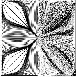
Figure 8: *Calculated (left) and observed (right) particle tracks underneath the cooled lid (plane  $y=0.95$ ) viewed from above.*
