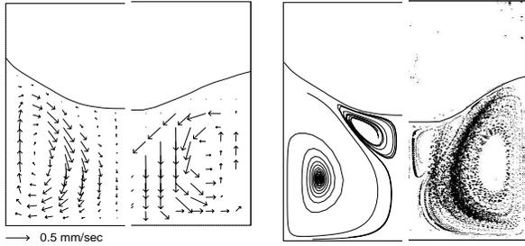
Figure 11: *Calculated (left half) and measured (right half) velocity vectors and particle tracks at the vertical centre plane  $z=0.5$ ;  $Ra = 3.1 \times 10^6$ ,  $Pr = 13$ .*
