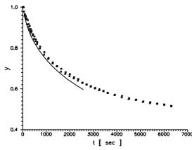
Figure 10: *Measured (symbols) and calculated (line) ice interface growth rate.*
