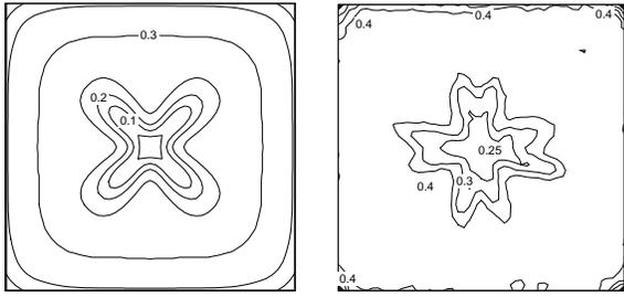
Figure 7: *Calculated (left) and measured (right) non-dimensional temperature distribution underneath the cooled lid (plane  $y=0.9$ ); water,  $Ra = 2.7 \times 10^6$ ,  $T_h = 21^\circ C$ ,  $T_c = 15.5^\circ C$ , steady state.*
