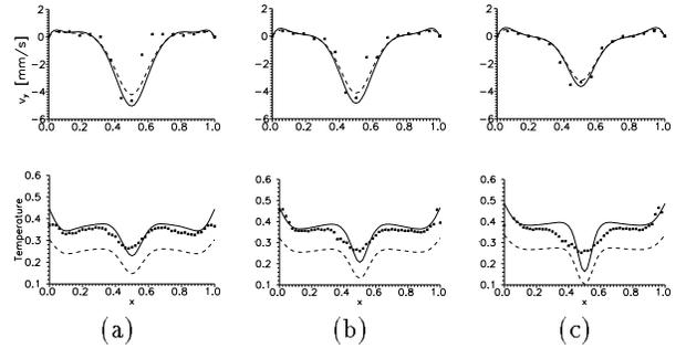
Figure 6: Comparison of velocity (above) and temperature (below) profiles for the final state at the  $z=0.5$  and (a)  $y=0.25$ , (b)  $y=0.5$  and (c)  $y=0.75$ . Measured values (symbols), calculated profiles using nominal heat flux (dashed lines) and fitted one (full lines).
