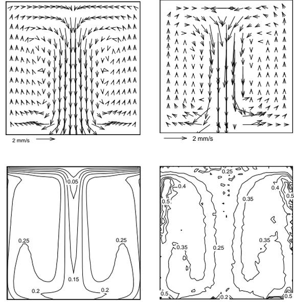
Figure 5: Convection in the lid-cooled cavity at the vertical symmetry plane  $z=0.5$ . Velocity and non-dimensional temperature at the final state ( $t=60$  minutes). Numerical simulation (left); experiment (right).
