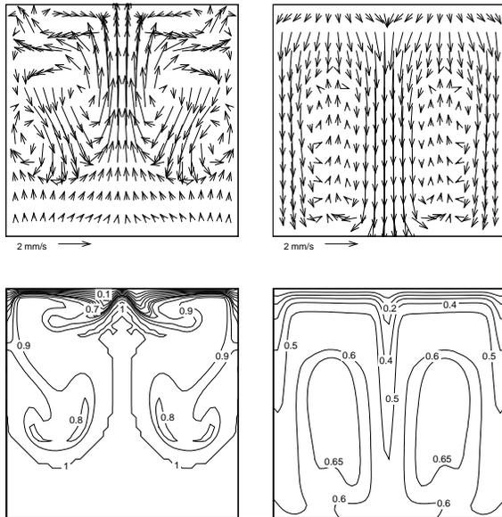
Figure 2: Onset of convection in the lid-cooled cavity.  $Ra = 2.7 \times 10^6$ ,  $Pr = 8$ . Numerical simulation for  $t=40s$  (left) and  $t=200s$  (right). Velocity vectors and non-dimensional temperature at the vertical centre plane  $z=0.5$ .
