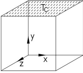
Figure 1: *The cubical box with cooled top surface. The y-axis is parallel to the gravity vector  $\vec{g}$ .*
