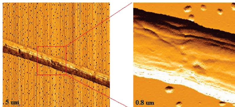
**Figure 1.** AFM picture of the BSA fiber reinforced with the addition of 15% PEO. The fiber width is nearly 400 nm. AFM height profile of this fiber indicates the thickness of the fiber to be only 73 nm. The scale corresponds to the image width (AFM scan size).
