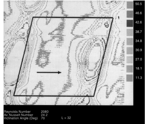
Fig. 15. False colour image of local Nusselt number contours over a central diamond of the undulated plate of corrugated-undulated geometry ( \phi=70^\circ , Re=2080 , H=8.8\text{mm} , L=32\text{mm} ).
