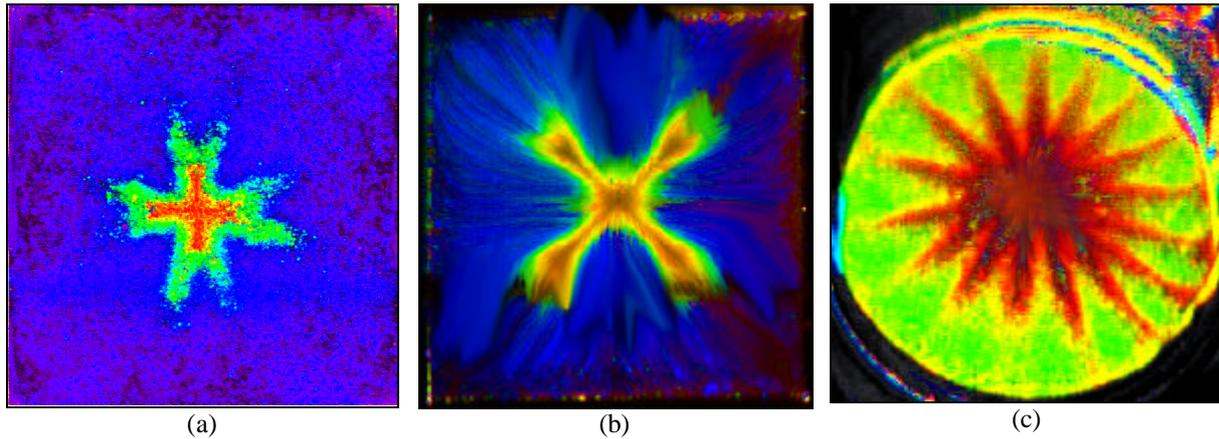
**Figure 6.** Natural convection in the lid cooled cavities. Temperature distribution recorded with help of TLC directly under the cooled top wall. Effect of the walls properties on the flow structure visible in the temperature fields: (a) - plexiglas walls, (b) - glass walls, (c) - cylindrical glass cavity
