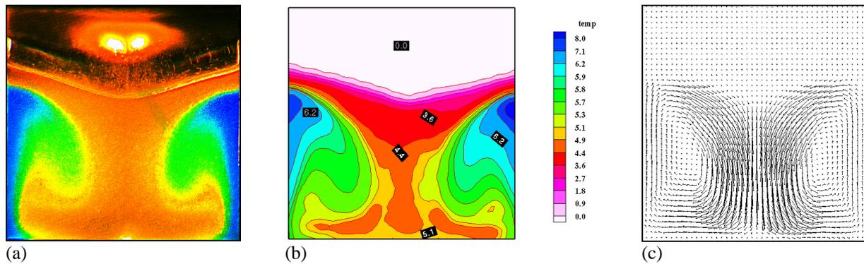
**Figure 5** Modeling crystal growth; freezing of water from the top in the lid cooled cavity. Recorded image of TLC tracers (a), evaluated temperature (b) and velocity (c) fields. Time step - 3600s after cooling starts; Isothermal lid temperature  $T_c = -10^\circ\text{C}$ , external bath temperature  $T_{\text{ext}} = 20^\circ\text{C}$ .
