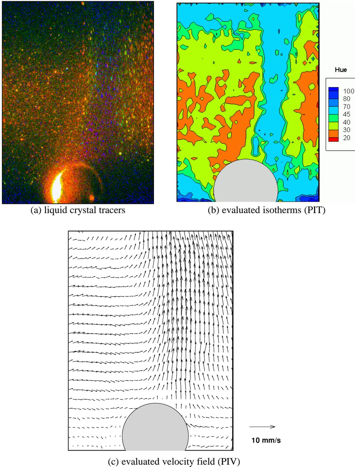
**Figure 8.** Flow field surrounding the steady vapor bubble visualized with liquid crystal tracers; evaluated temperature field (b) and velocity field (c);  $P = 6.1 \text{ kPa}$ ,  $T_l = 35.7^\circ \text{C}$ ,  $T_b = 57^\circ \text{C}$
