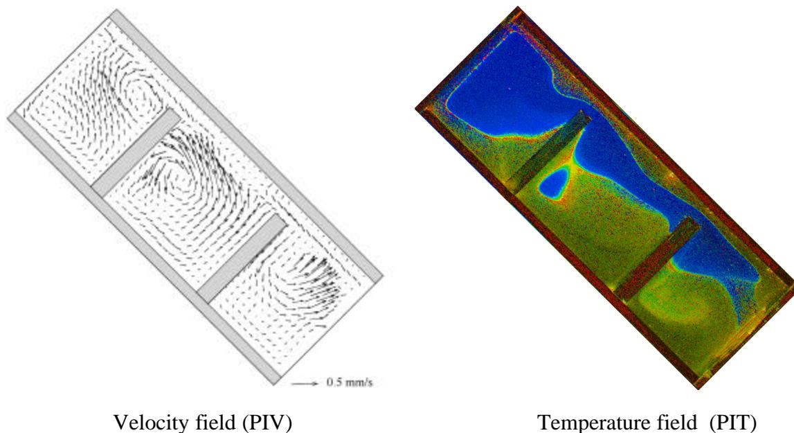
**Figure 7.** Velocity field and temperature distribution visualized for the cavity inclined under  $45^\circ$ . Two cold isothermal walls (upper and lower) are responsible for sudden cooling of the fluid. It changes colour of the liquid crystals seeding from blue (hot) to red (cold regions).
