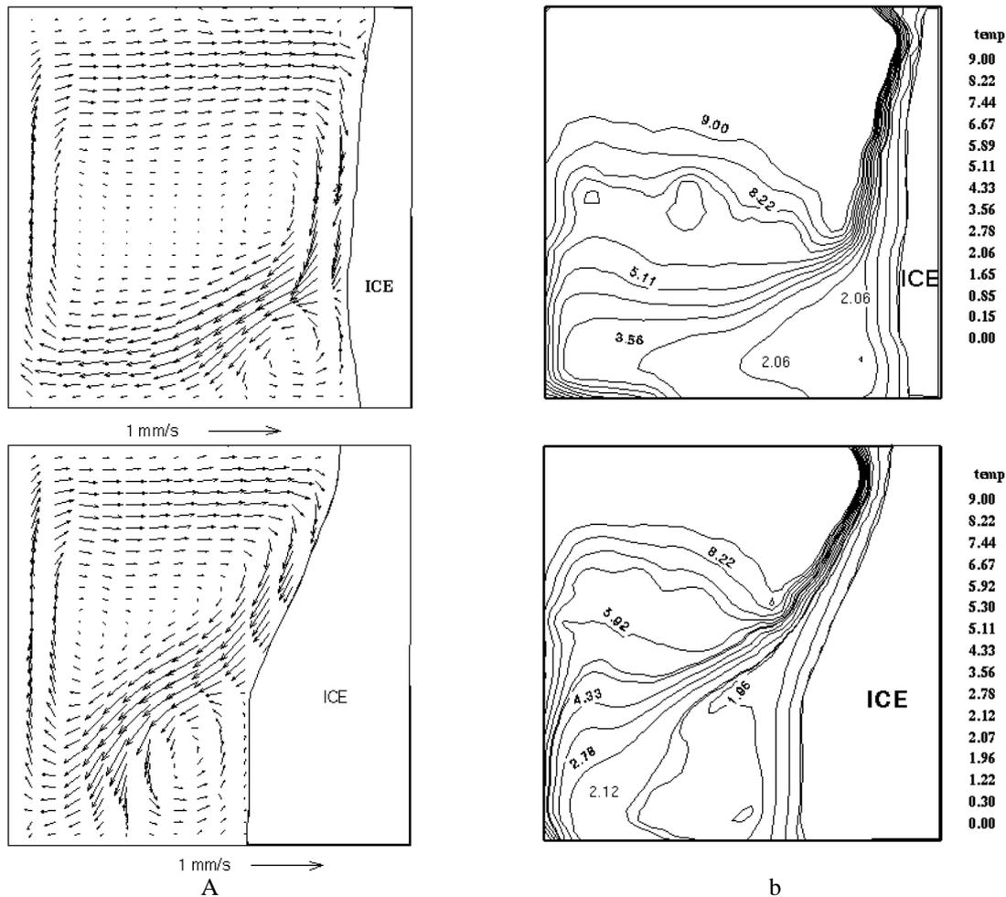
**Figure 4.** PIV (a) and PIT (b) measured velocity and temperature fields for natural convection in center plane of differentially heated cavity at 500s (top) and 3000s (bottom).  $T_h=10^\circ\text{C}$ ,  $T_c=-10^\circ\text{C}$ ;  $Ra=1.5 \cdot 10^6$ ,  $Pr=13.3$
