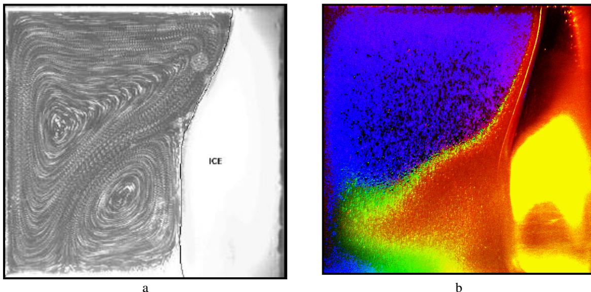
**Figure 3.** Modeling directional solidification; water freezing in a differentially heated cube shaped cavity. Particle tracks showing flow structure (a), liquid crystals tracers indicating variation of temperature (b). Left hot isothermal wall at  $T_h=10^\circ\text{C}$ , right cold isothermal wall at  $T_c=-10^\circ\text{C}$ .
