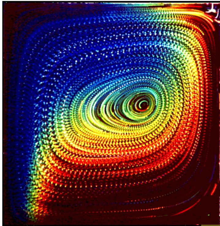
**Figure 1.** Multiexposed color photograph of the convective flow in glycerol seeded with liquid crystal tracers in a differentially heated cavity. Tracers change color from blue to red following the clock-wise flow circulation from the hot wall (left) to the cold wall (right); temperature difference  $\Delta T=4^\circ\text{C}$ .
