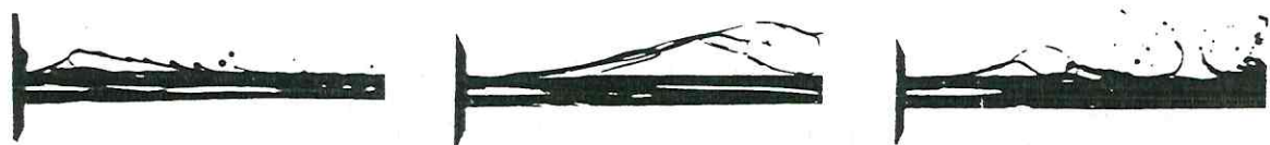
Fig. 6 - Ethanol jet, D = 200 \mu\text{m} , V = 12 \text{ m/s} , P_\infty = 100 \text{ Pa} , P_s = 5.9 \text{ kPa}
