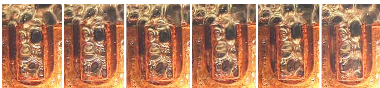
Figure 9. Water boiling internal visualization at high heat flux ( q \approx 230 \text{ kW/m}^2 ), frames every 0.005 s.
