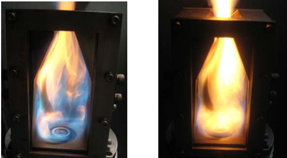
Fig. 4 Direct photographs of spray flame for fuel-lean (left) and -rich (right) combustion
