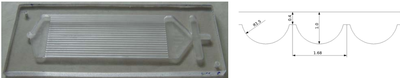
Figure 2. Left: experimental channel with 20 spanwise wall corrugations. The top wall is flat for better optical access; right: cross section of the channel with dimensions of the corrugations (in mm).
