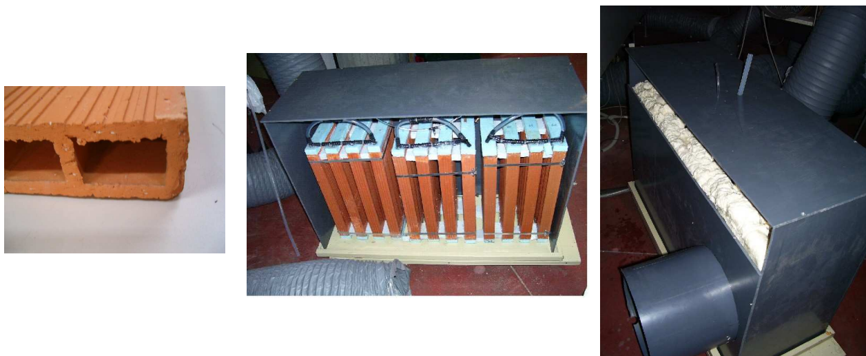
Figure 3. Semi-indirect Ceramic Evaporative Cooler (hollow bricks).
