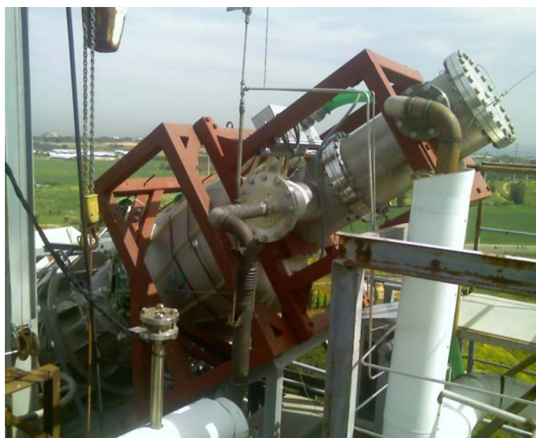
Figure 5: The SOLREF reactor installed on the WIS solar tower.
