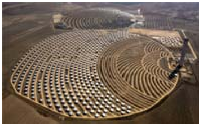
Figure 4: First commercial solar tower power plants PS-10 in operation and PS-20 under construction (Seville, Spain).
