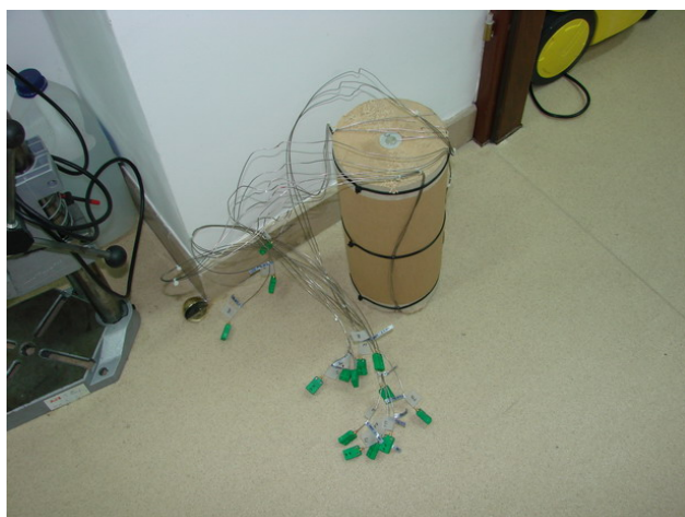
Figure 11. The paper coil equipped with thermocouples
