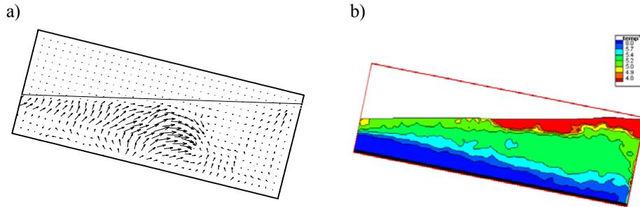
Fig. 1. Water filling cavity and freezing at the side walls after 20s: a) PIV evaluated velocity field; b) PIT evaluated isotherms. Inclination  $\alpha = 78.6^\circ$ ,  $T_c = -15^\circ\text{C}$ ,  $T_h = 3^\circ\text{C}$ ,  $Q = 4.6 \cdot 10^{-6} \text{m}^3/\text{s}$
