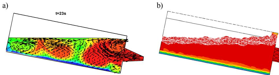
Fig. 2. Numerical simulations of the case from Figure 1: a) temperature and velocity fields from Fluent, b) fluid surface and temperature distribution from Procast
