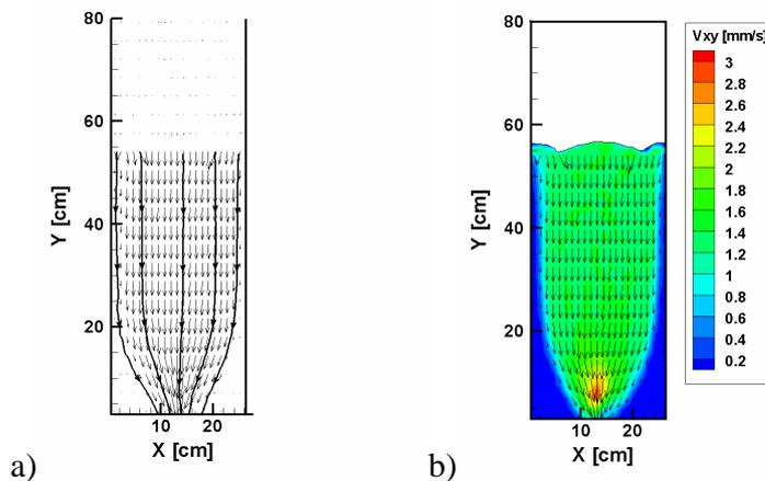
Fig. 3, Central discharge, amaranth seed, medium rough walls, a) vector field, b) velocity magnitude contours for the 15<sup>th</sup> second of the flow
