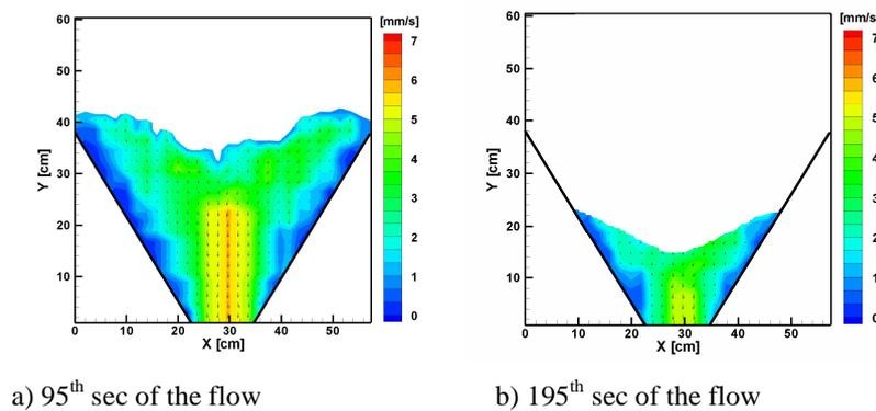
Fig. 6, Velocity magnitude contours for flowing amaranth at 95<sup>th</sup> and 195<sup>th</sup> sec of the flow
