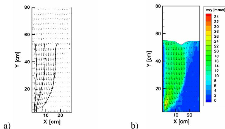
Fig. 1, Eccentric discharge from the left, amaranth seed, medium rough walls, a) vector field, b) velocity magnitude contours for the 30<sup>th</sup> second of the flow
