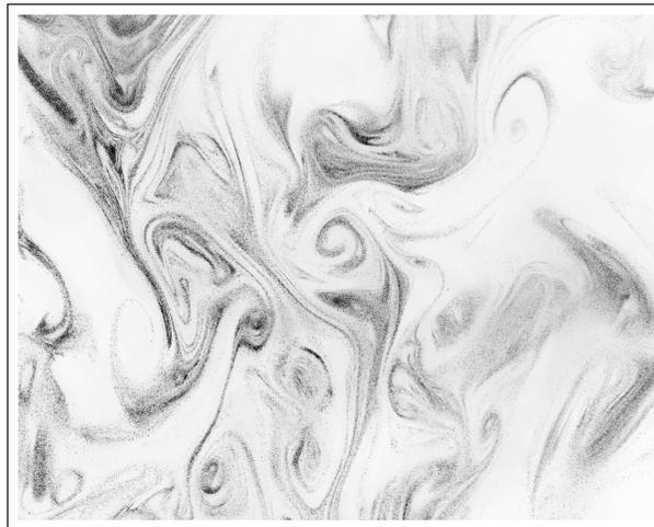
*Fig 2:* The negative of the cloud image from the experimental chamber showing small-scale structures created in a process of cloud-clear air mixing. Imaged area corresponds to  $7\text{cm} \times 4.5\text{cm}$  in physical space.
