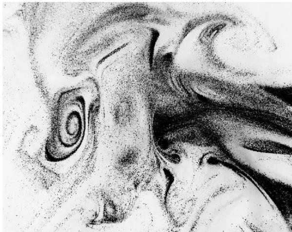
Fig.1. An example image from the cloud chamber. Dark pixels are occupied with cloud droplets. Image covers area of  $\sim 9 \times 6 \text{cm}^2$
