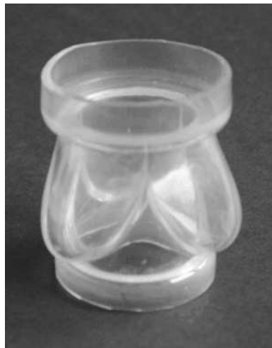
FIGURE 10. 10:1 model of a polyurethane tri-leaflet valve
