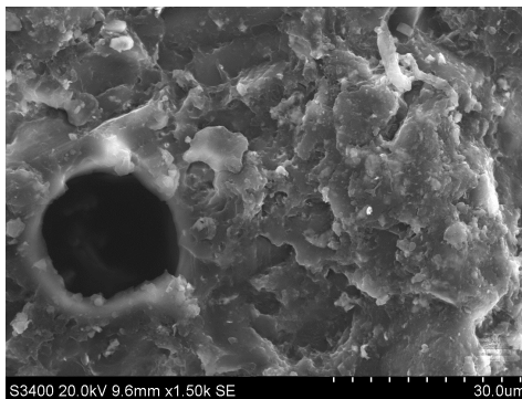
Fig. 2 SEM images of fracture surfaces, epoxy resin without filler a) and epoxy resin with nanofiller b)
