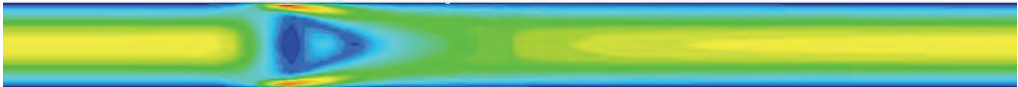
Fig. 1. Velocity field maldistribution for the paramagnetic fluid flow in the strong magnetic field
