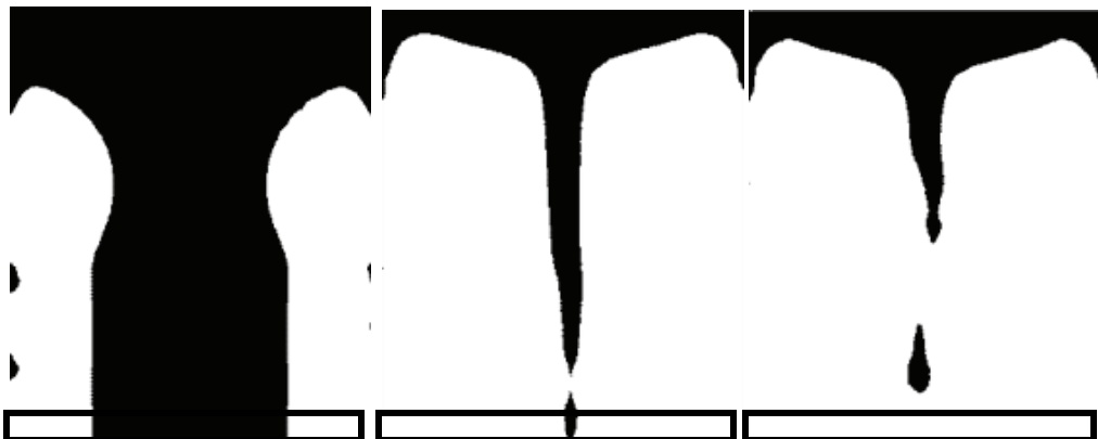
Fig. 1. Rivulet flow structure formed at the subcritical Reynolds number regime – temporal evolution
