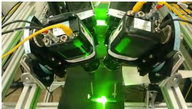
Volumetric PIV, 4 cameras, 1 kHz real-time
