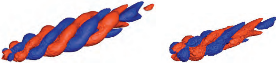
Fig. 1. Real parts of Complex Dynamic Response modes for a time-averaged flow past a sphere at Re = 400 , St = 0.134 and two different real parts of complex shift
