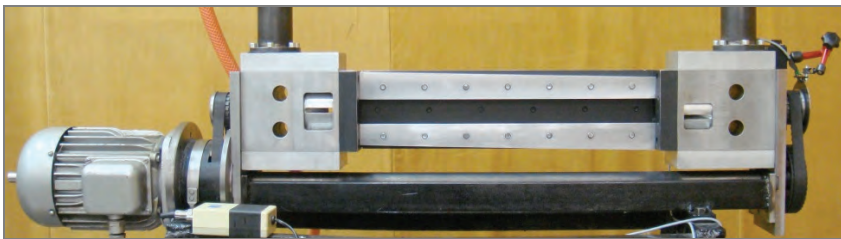
Fig. 2. The examined pressure wave exchanger with revealed flow channel
