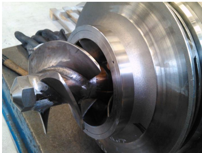
Fig. 1. View of the three blade inducer of the studied pump
