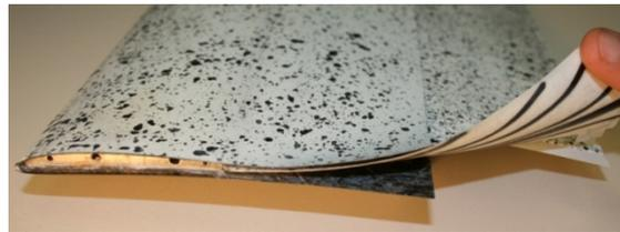
Fig. 2 Flexible airfoil
