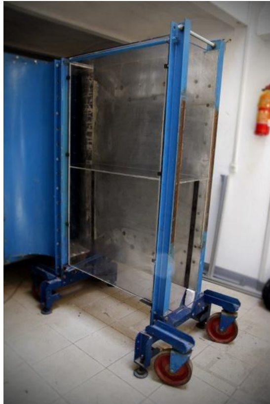
Fig. 3 New test section with plexiglass walls
