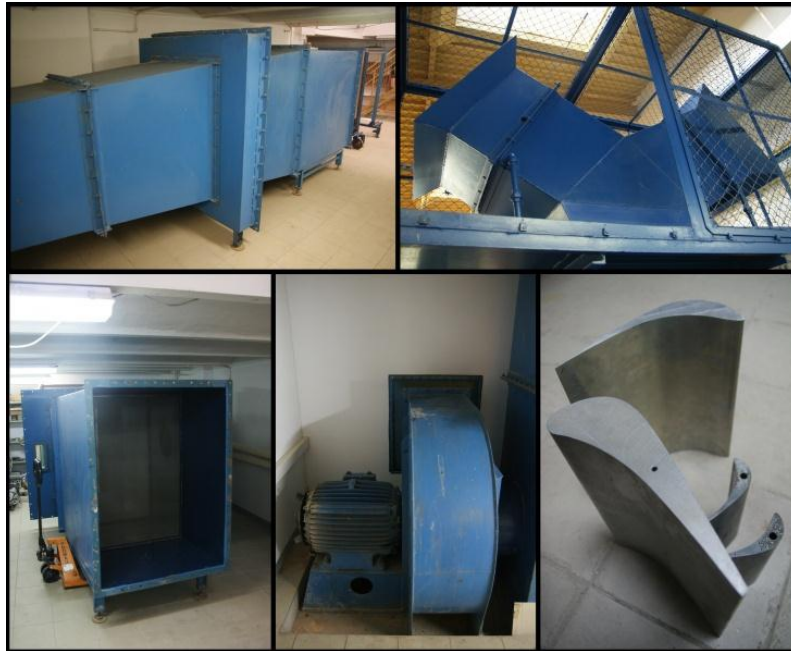
Fig. 2 Present-day overview of IMP WT; from top-left clockwise: 1. diffuser, suction chamber and flow stabilisation section; 2. inlet channels with cooling system; 3. examples of tested blades; 4. powering engine-fan unit; 5 outlet from flow stabilisation section (grids visible)
