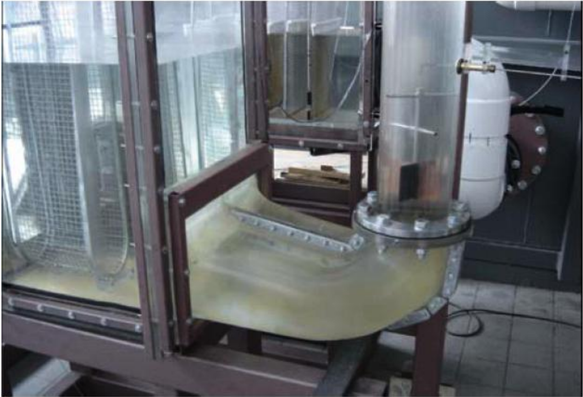
Fig.2 View of the model of the cooling water pump suction intake
