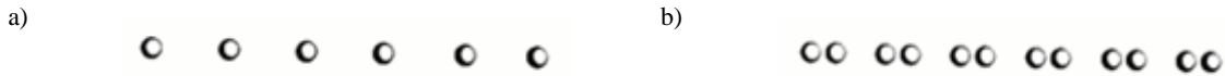
Rys. 1 Sample Picture for measurements of a) Droplets evaporation, b) droplets velocity measurements
