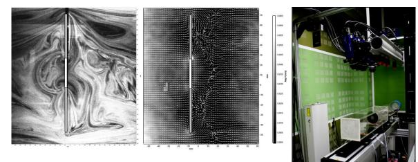
**Fig. 1.** PIV experimental setup (right) with sample particle image (left) and processed acoustic particle velocity field map (centre)
