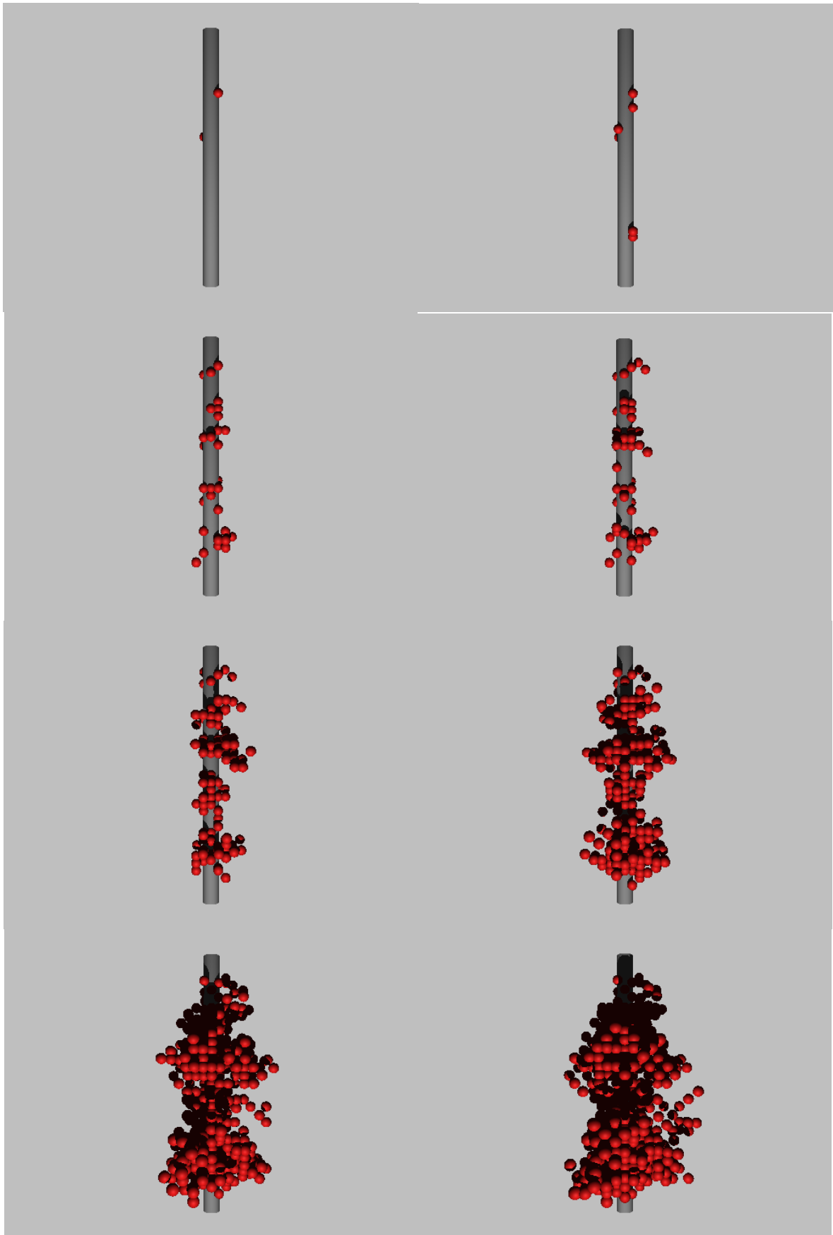
Fig. 1 Stages of dendrite growth (view from the upflow).
