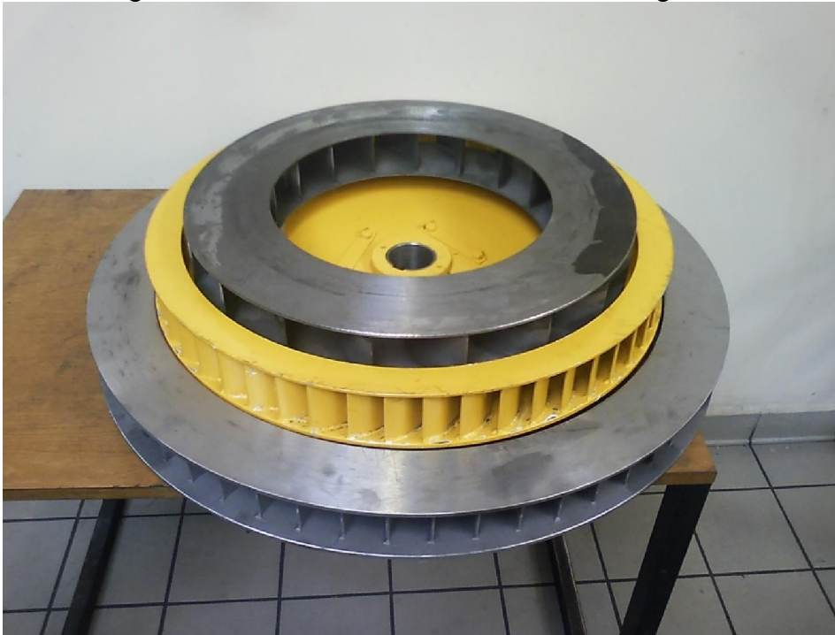
Photo 1. View of the model blading blower, geometrical variant D.
