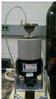
Figure 1 Surface mechanical attrition treatment (SMAT) Setup
