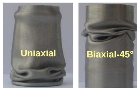
Fig. 2 Typical examples of the deformation modes for the specimens having \eta = 15.5 under different dynamic loading complexities.
