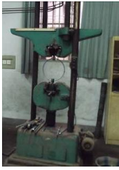
Fig.7 Tensile test on a single wire ring
