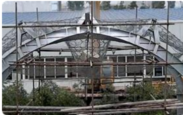
Fig.10 The flexible rock shed deformation obtained by the numerical simulation and the test when the rock-fall falls in the lowest point
