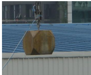
Fig.6 Concrete block for impact test
