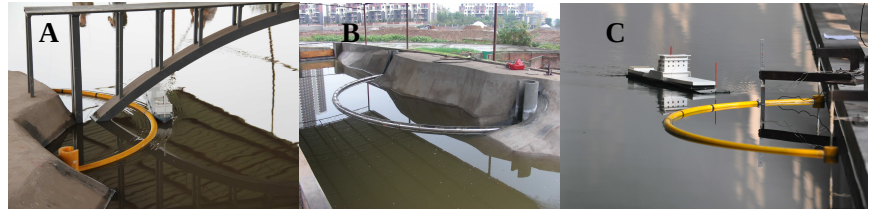
Fig.5.A. 1:100 model experiment in the dynamic water .B. 1:25 model self-operation status experiment C. static water collision experiment
