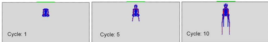
Fig. 1 Damage patterns at different thermal shock cycles (0,5 s heating + 2 s break), green: surface heat flux 42 MW/m 2 , blue: pre-damage area, red: destroyed domains/ macrocrack
