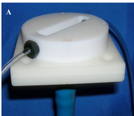
Figure 1. Optical image of custom fabricated device used to mechanically stimulate cells (A) and schematic of single cells experience multiple modes of mechanical stimulation (B).
