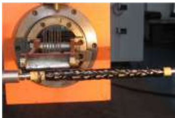
Fig. 1 Filament wound of F 2 MC tube
