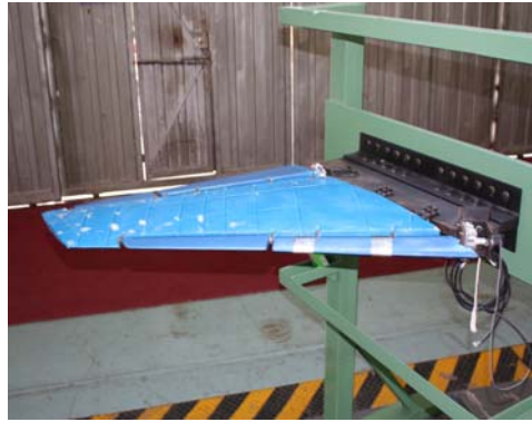
Fig. 1 The wind-tunnel model of a wing equipped with four control surfaces
