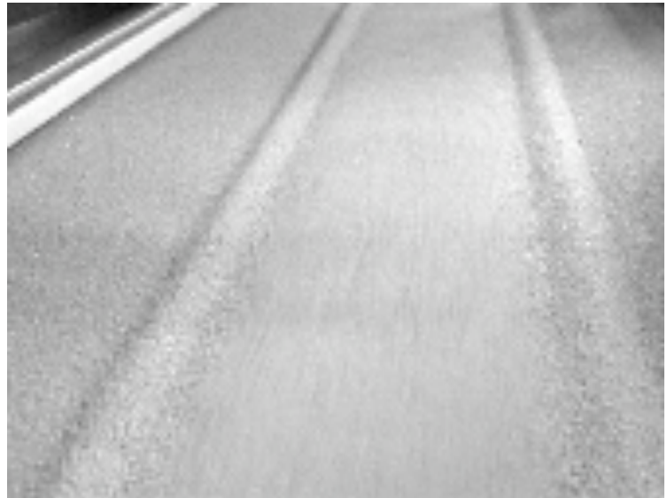
Figure 1: Photograph of the experimental set up (left) and steady channel of flowing sand confined by levees (right).
