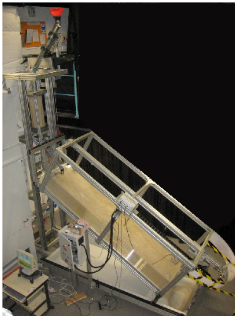
Figure 1: Photograph of the experimental set up (left) and steady channel of flowing sand confined by levees (right).
