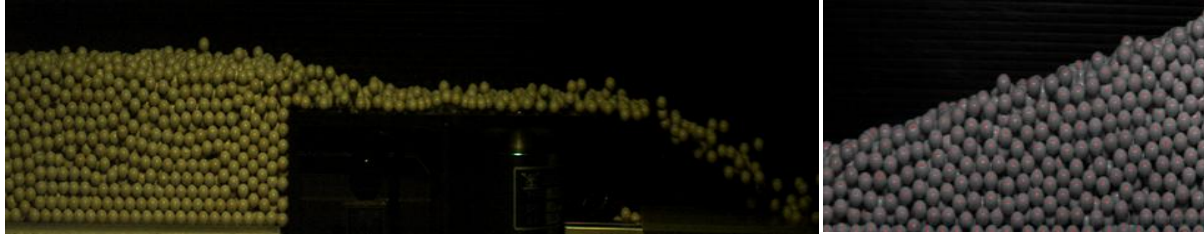
Figure 4: (left) Snapshot of the granular flow over the sensing module; (right) the sphere located by circular Hough transformation method.
