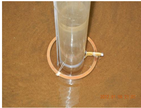
Figure 3: Circular Cylinder Pier Model with Control Ring Attached.
