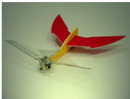
Fig. 1. The 20 cm-span flapping MAV “Golden Snitch”[2]. Fig. 2. Figure-of-8 wingtip trace of “Golden Snitch”[1,3].
