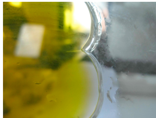
Figure 1. Surface profile obtained with the theory of perturbation applied to the stream-function. Note the asymmetry. Cusp exhibited in a swelling gel experiment in the circular geometry.
