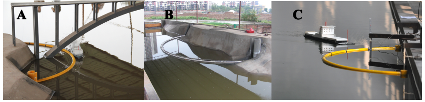
Fig.3. A. 1:100 model experiment in the dynamic water .B. 1:25 model self-operation status experiment
