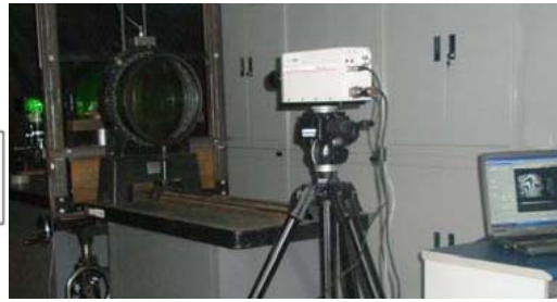
Fig.2 new-type dynamic photoelastic system
