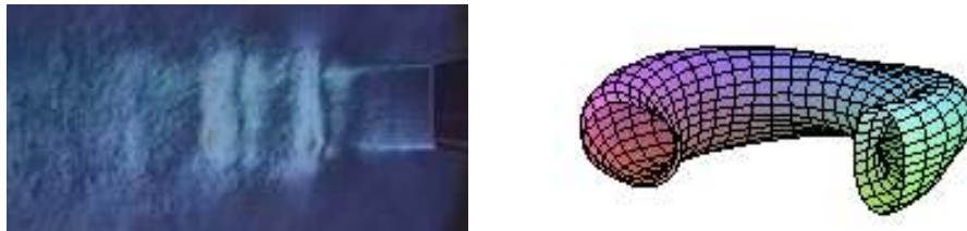
Fig. 1. In the tone excited jet large vortex structures are identical to a vortex ring train (a), radiating mode of vortex ring accompanied by rotating deformation of vortex core (b).
